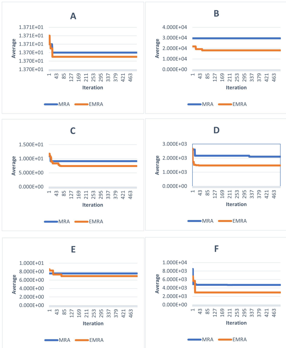
Figure 2: Convergence behavior of EMRA and MRA over iterations for the CEC2019 functions, where (A) corresponds to F3, (B) to F4, (C) to F5, (D) to F7, (E) to F8, and (F) to F9.
