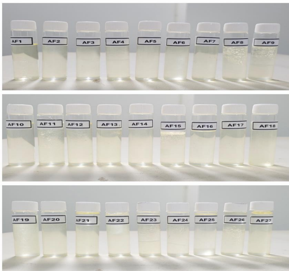
Figure 5: Zavegepant-loaded microemulsion batches prepared through Central Composite Design, illustrating the systematic optimization of formulation variables to evaluate their influence on globule size, zeta potential, polydispersity index, viscosity, pH, mucoadhesive strength, and drug content.
